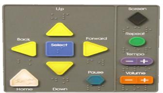
Figure 19 - Keypad of the Ballot Marking Device
