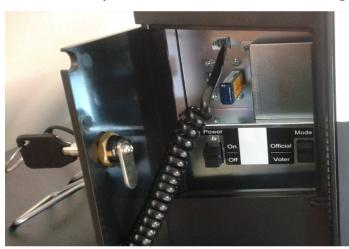
5. Flip the "Power" switch to the "Off" position.
